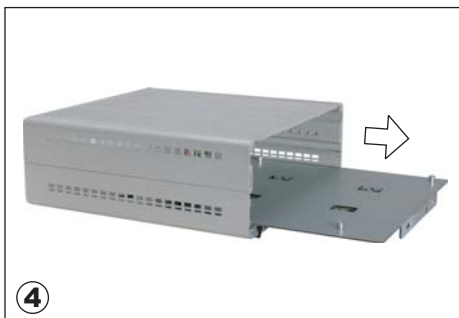
Take the HDD cage out of the chassis.
