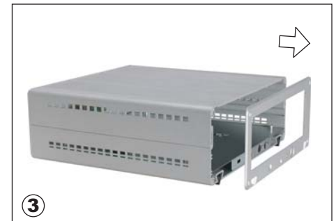
Take the back panel out of the chassis.
