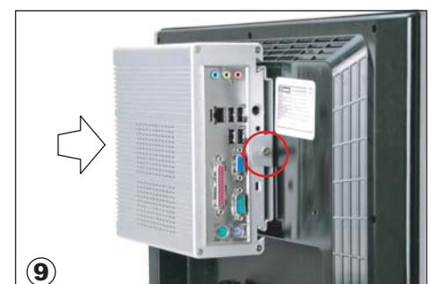
Fix 1 screw on the back of monitor.
